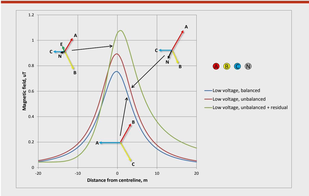
\*Note: Hypothetical examples. Actual field levels will depend on specifics of the powerline, nature of the loading and earthing system. Calculations include only 50Hz currents and assume the electrical angles between the three phases are 120 degrees.
