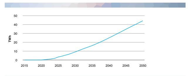
**Figure 13:** Projected additional national aggregate non-coincident zone substation load from predominantly unmanaged electric vehicle charging
