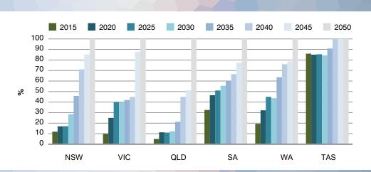
**Figure 30:** Projected ratio of battery capacity to variable renewable generation capacity to achieve energy balancing for a given renewable energy share, by state.
