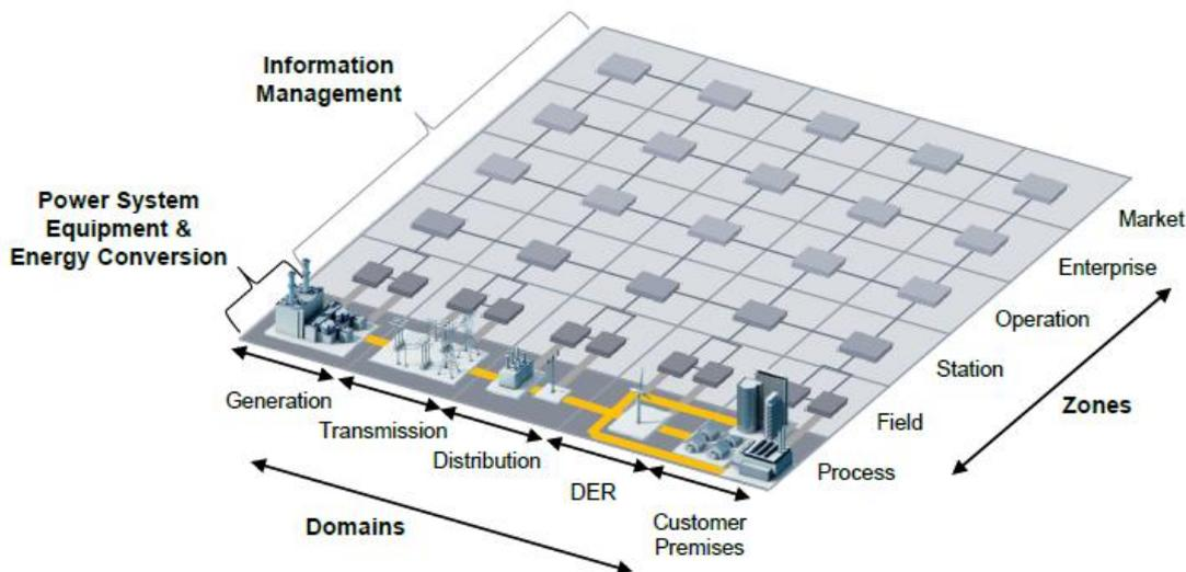
Figure 7: Smart Grid plane - domains and hierarchical zones
