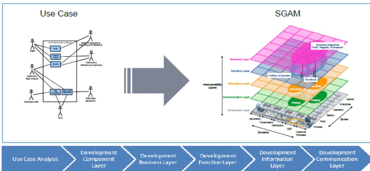
**Figure 12: Use case mapping process to SGAM**
