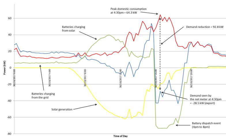
Net meter power, solar power, battery power and domestic power for one of the battery dispatch events during summer 2017/18 period
