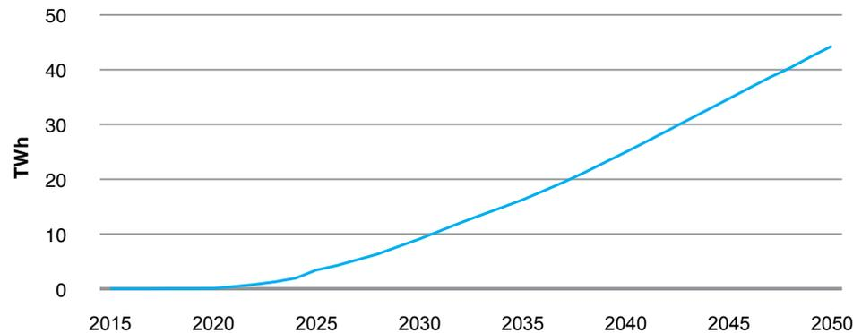
**Figure 13:** Projected additional national aggregate non-coincident zone substation load from predominantly unmanaged electric vehicle charging
