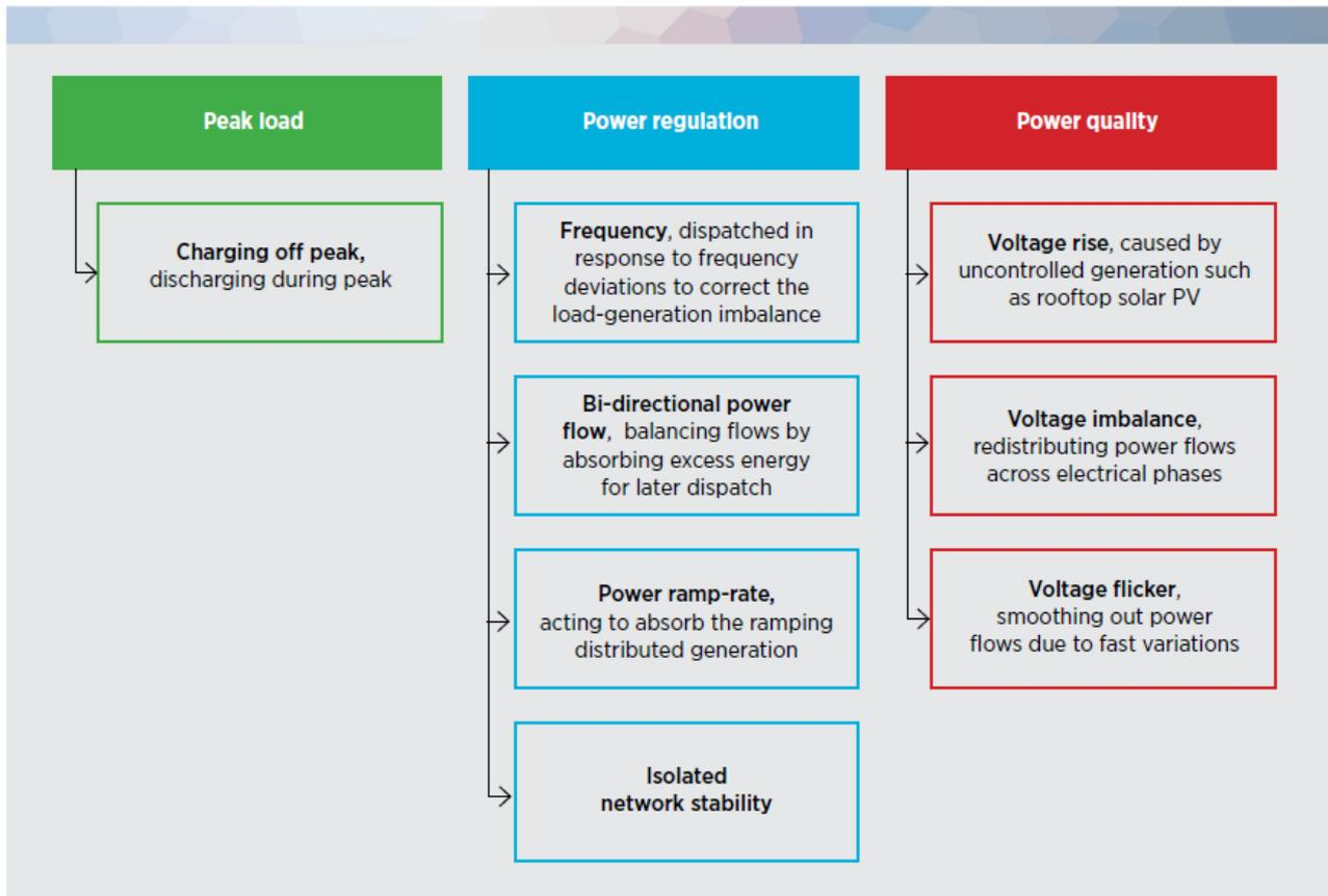
Figure 3 How Storage Can Accommodate DER [REF: Energy Networks Australia, 2015, “Electricity Network Transformation Roadmap, Interim Program Report”, Pg. 77.]
