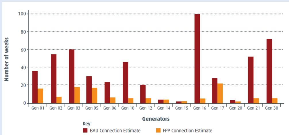
Time to connect a generation customer, comparing BAU with FPP offers.
