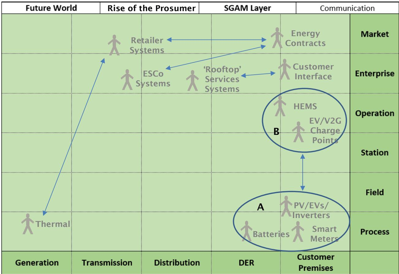
Figure 18 Rise of the Prosumer - SGAM Communication Layer
