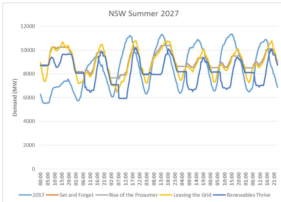
Figure 2 New South Wales summer demand in 2017 and 2027 (based on data from CSIRO)
