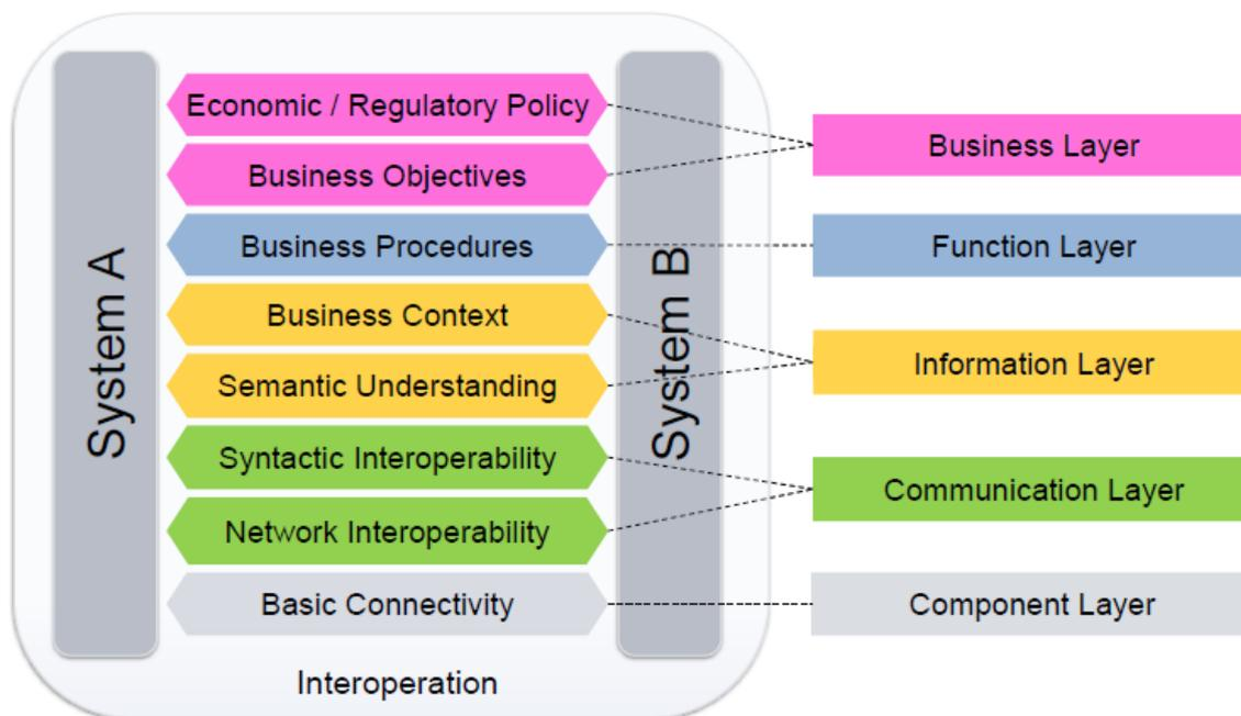
**Figure 6: Grouping into interoperability layers**
