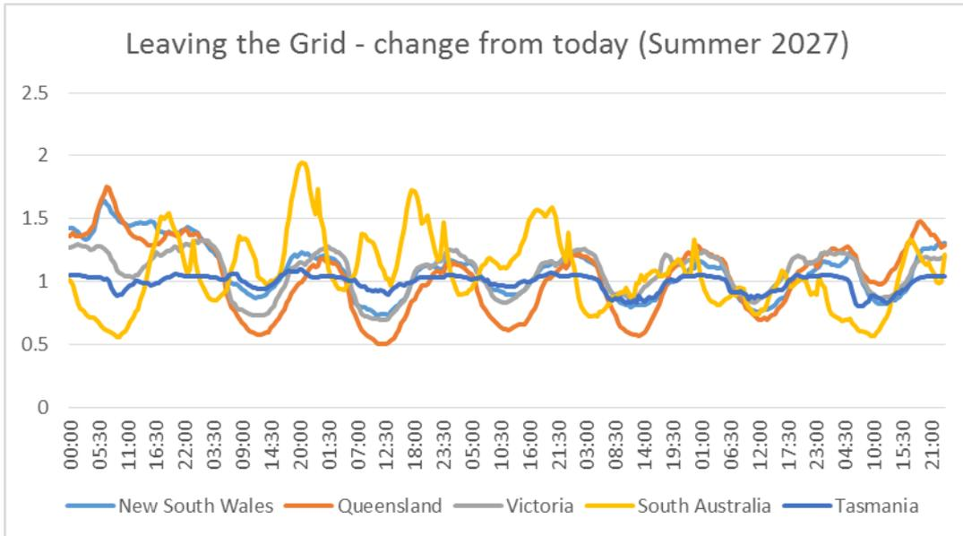
Figure 4 Expected demand by state in 2027 under the Leaving the Grid scenario (data from CSIRO)
