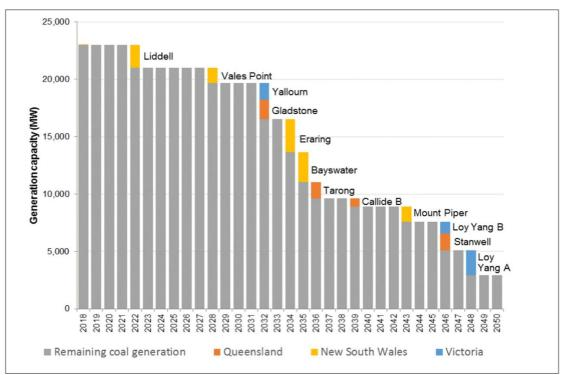
Figure 5: NEM coal generation fleet if plant retires as announced or at 50<sup>th</sup> year from full operation
