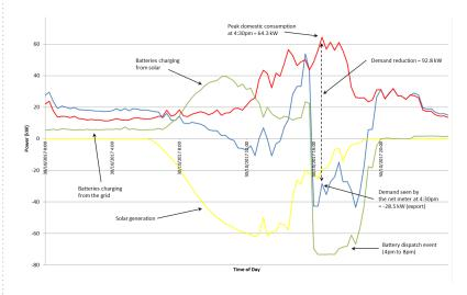
Net meter power, solar power, battery power and domestic power for one of the battery dispatch events during summer 2017/18 period
