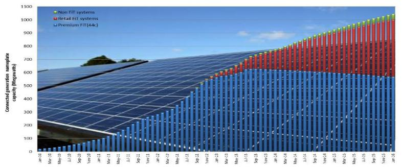
~1100MW on installed domestic PV capacity in a ~5000MW network. In some postcodes >40% of customers have PV. Total energy delivered is ~7% (1438GWh) of total
