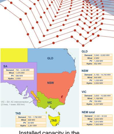
Installed capacity in the NEM
