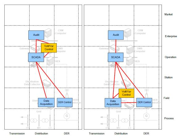
Figure 17: Flexibility for assignment of function "Volt/Var Control" to SGAM segments, case A - in operation zone, case B - in field zone
