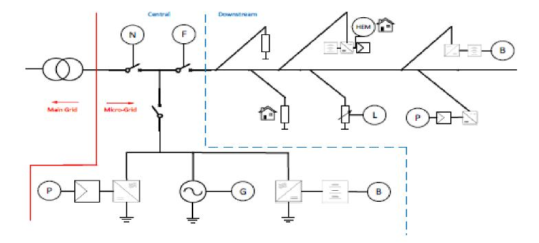
The generic model of a Microgrid/minigrid could contain any or all of the following components or power assets that can be deployed, started up, shut down, connected or disconnected multiple times a day and/or have continuously controlled power generation or consumption
